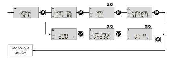
The S2Ca can also run in calibration mode. The corresponding continuous displays show the current dosing quantities or the feed rate.
